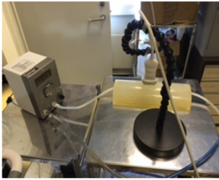
Fig 1. Pulsatile flow-simulating phantom design for the measurement's accuracy.
