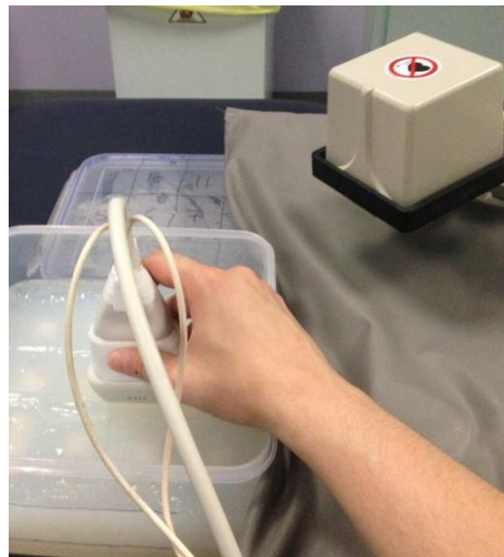
(Figure 3. Magnetic tracking box and tracking sensors of a 3D free-hand sensor tracked system)
